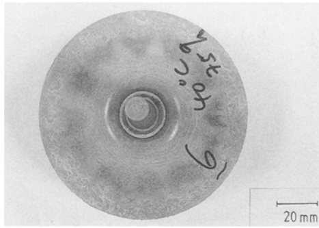
Figure 7 Moulding made at 40°C mould temperature using oscillating pressure.
